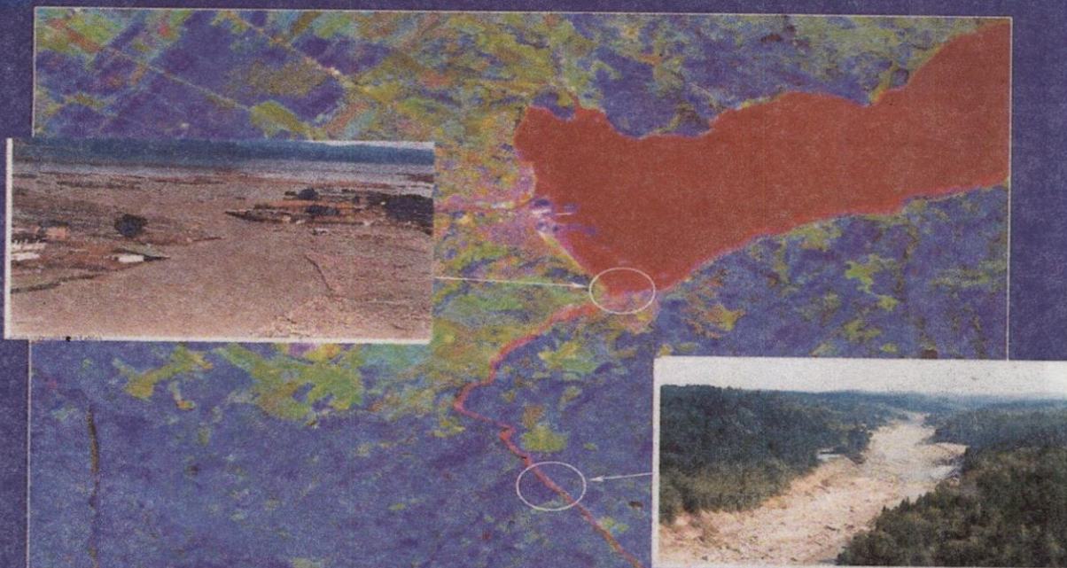
Color composite image showing Landsat Thematic Mapper channel 2 data acquired on July 29, 1996 (red), June 27, 1996 (green), and Radarsat Fine Beam 4 on August 9, 1996 (blue). Red areas are exposed or suspended sediment as a result of the flood event.
