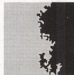
Figure 4: the result of applying iterative region-merging to the output of the pixel based maximum likelihood classification.
